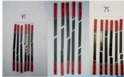
Figure 33. Typical failed specimens. Source: Author.
