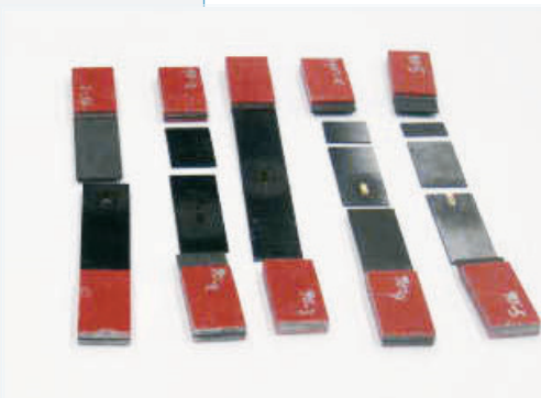
Figure 19. 90° specimen failed. Source: MSE 597 report
